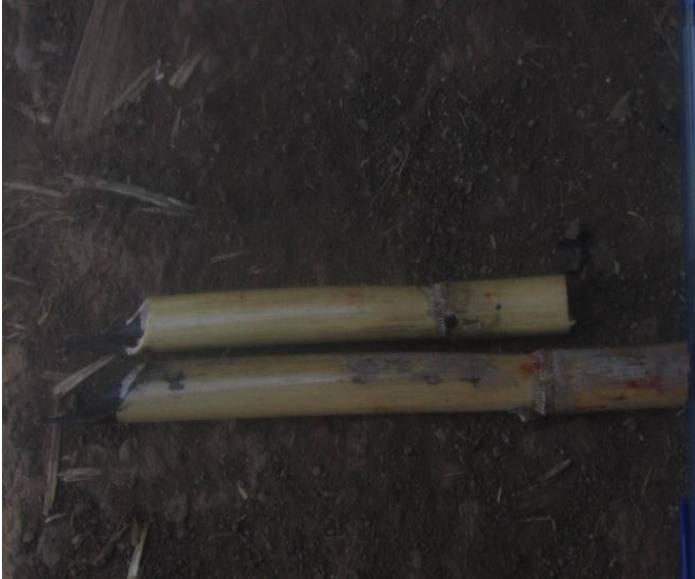
Fig.8.the red ink pen (left) and black ink pen (right) made from bamboo
